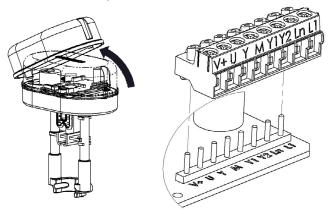
The actuator is equipped with a 8 poles removable terminal block; each pole of the plug is clearly marked and the same label are reported on the electronic board. Before powering up the actuator make sure the plug is properly connected to the board and the label on the plugs and on the board match.
